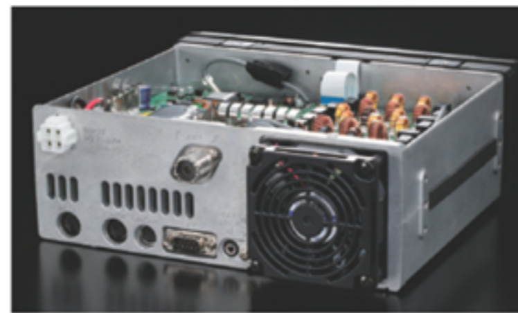
The rugged aluminum die-cast chassis with cooling fan
